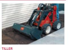
Hardened steel tines for any soil condition, including clay or hardpan. Till more than six inches deep and 40" wide on one pass. Reversible tine direction frees jams quickly.
