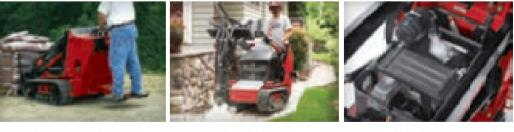
LOW-IMPACT FOOTPRINT Long-lasting, Kevlar<sup>®</sup> reinforced Quickly and easily bolted on to tracks disperse weight evenly for a light footprint on turf, while this ride-on platform helps delivering better traction in sandy or wet ground conditions.
