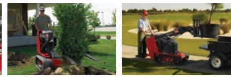
**TREE FORK** Hydraulic fork arm opens to handle large trees and shrubs. Angle design allows for gentle handling.
